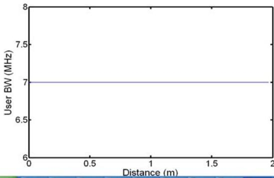
Figure 13 User Bandwidth allocations for FDMA scheme
