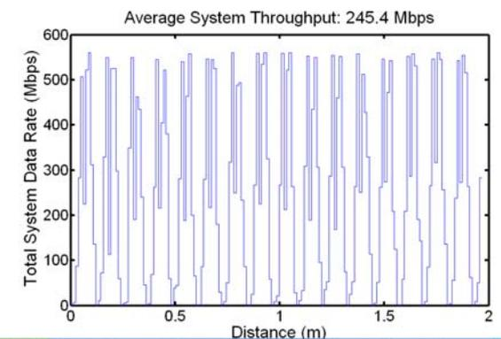
Figure 6 Average system throughput for TDMA user bandwidth allocation scheme
