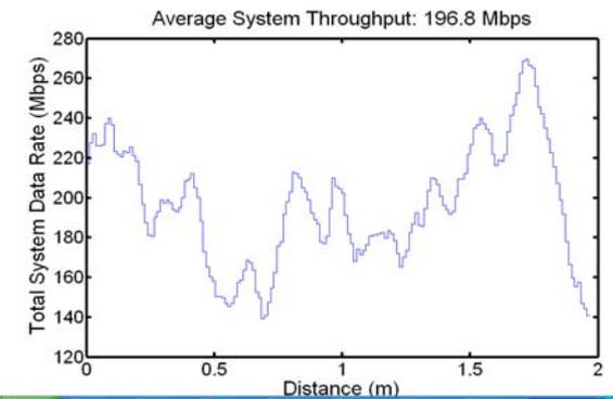
Figure 5 Average system throughput for FDMA user bandwidth allocation scheme
