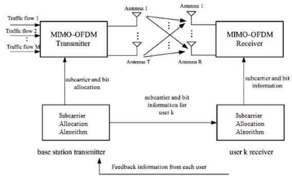
Figure 1 Bloch diagram of multiple antenna OFDM multicast system
