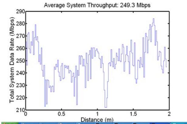
Figure 7 Average system throughput for Random user bandwidth allocation scheme
