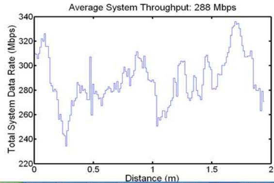
Figure 4 Average system throughput for Adaptive user bandwidth allocation MIMO-OFDM scheme
