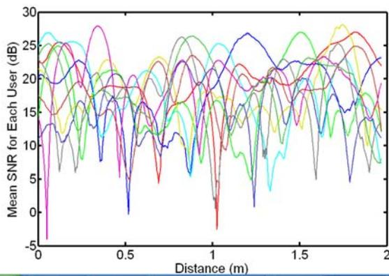
Figure 9 Mean SNR for individual user for FDMA user bandwidth allocation scheme
