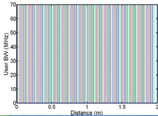
Figure 14 User Bandwidth allocations for TDMA scheme
