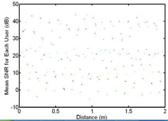
Figure 10 Mean SNR for individual user for TDMA user bandwidth allocation scheme
